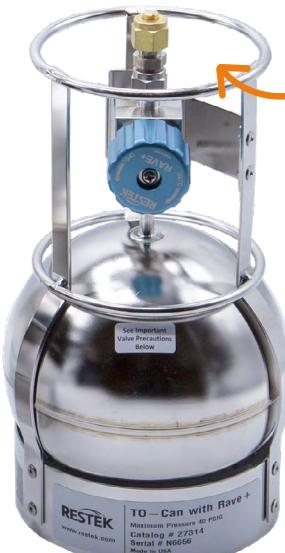
Do not overtighten the valve, and do not forget to replace the brass cap
